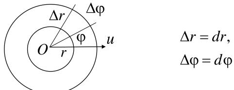
$$\Delta \sigma = \frac{1}{2} (r + \Delta r)^2 \Delta \varphi - \frac{1}{2} r^2 \Delta \varphi = r \Delta r \Delta \varphi + \frac{1}{2} \Delta r^2 \Delta \varphi \approx r \Delta r \Delta \varphi,$$
