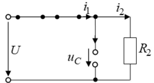
$$\begin{aligned} u_C(0) &= u_C(0_-) = U = 2 \text{ кВ}, \\ i_1(0) &= i_1(0_-) = U / R_2 = 2000 / 100 = 20 \text{ А}. \end{aligned}$$
