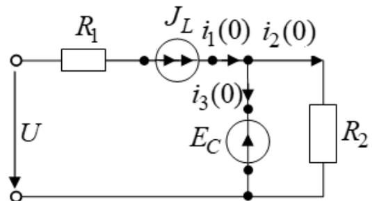
$$i_2(0) = E_C / R_2 = u_C(0) / R_2 = 2000 / 100 = 20 \text{ А}.$$
