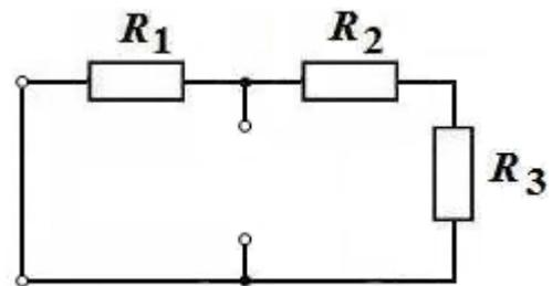
$$R_{\text{Э}} = R_1 (R_2 + R_3) / (R_1 + R_2 + R_3) = 50 (25 + 25) / (50 + 25 + 25) = 25 \text{ Ом.}$$
