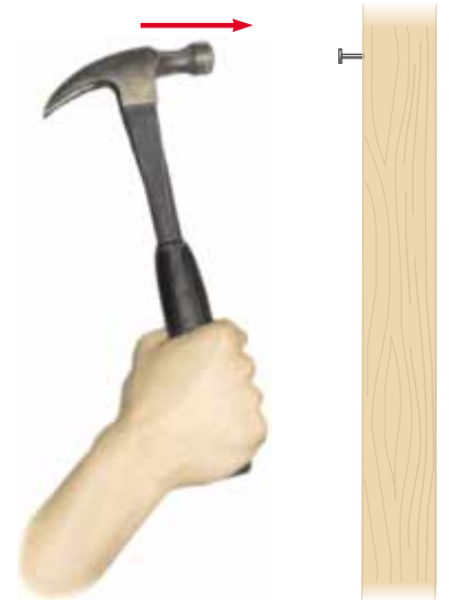
Figure 7.14 The moving hammer has kinetic energy and thus can do work on the nail, driving it into the wall.
